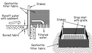
Geotextile Filter Fabric Drop Inlet Sediment Trap
