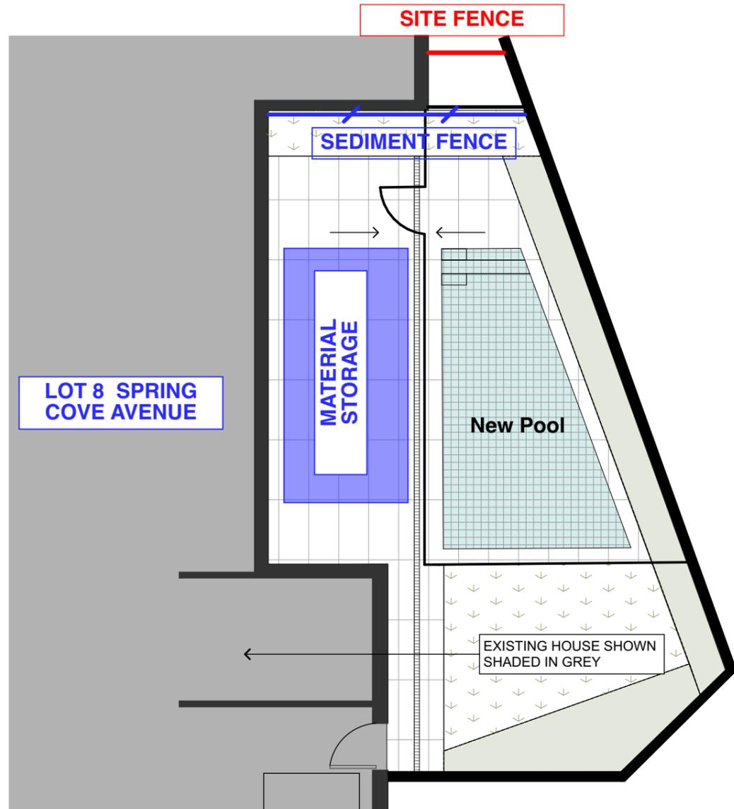
**Soil and Sediment Control Plan**
