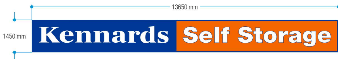
4A KENNARDS LANDSCAPE LOGO FRAME : BUILD OUT TO FIT IN FRONT OF PIPES SIGN PANEL : FOLDED BLUE ACM, PANELS OF EQUAL WIDTH : SIDE FIXED, NO FACE FIXINGS ALLOWED GRAPHICS : VINYL
