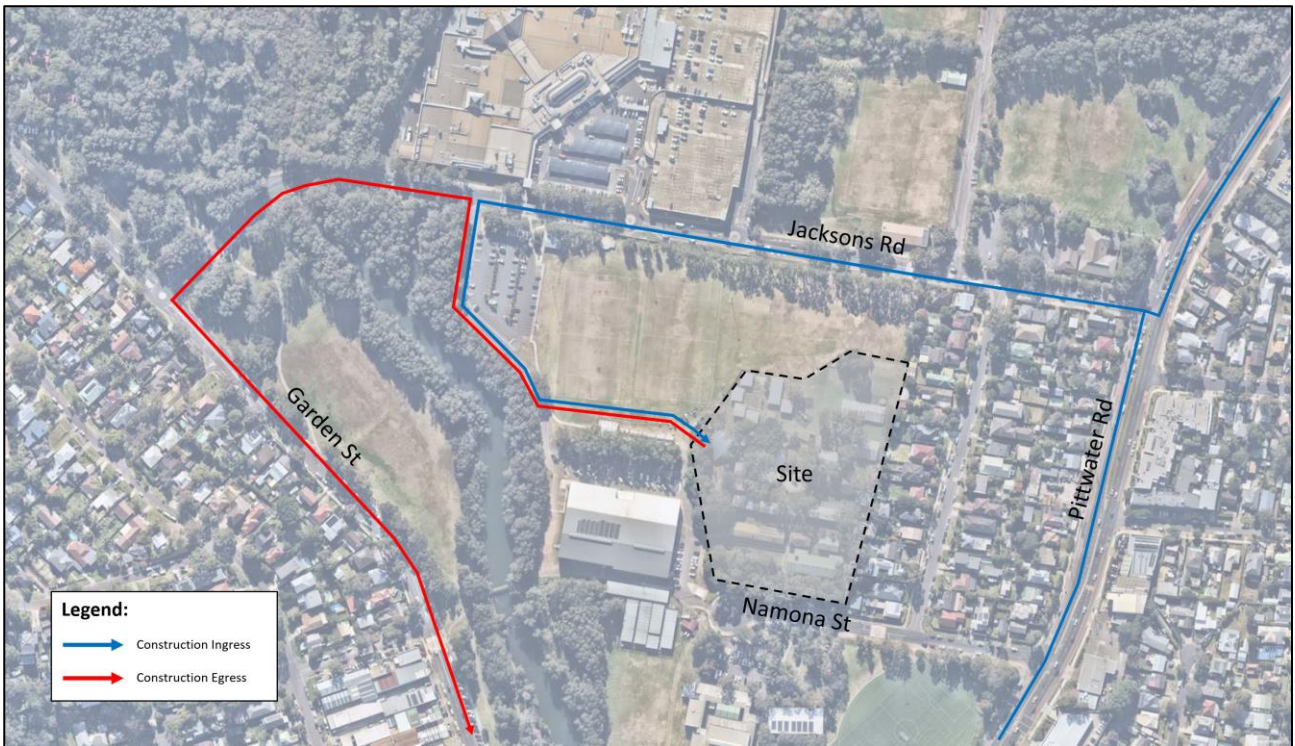
Figure 9: Construction Vehicle Haulage Routes
