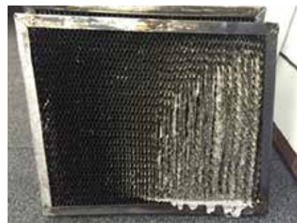
Figure 1: Heat of the fire melted the metal grease filter.
