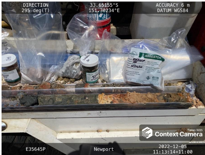
Photograph 1: Soil return from BH3
