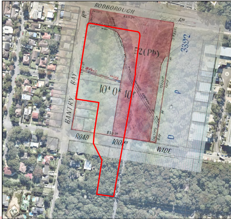
Figure 15: Extracted GIS plan from the RPS preliminary heritage assessment showing former drainage across the site. NOTE: the red curtilage in this plan is not the proposed development area but rather the project area relevant to the RPS report. Further, the original source map was not identified as no source reference is provided in the report.
