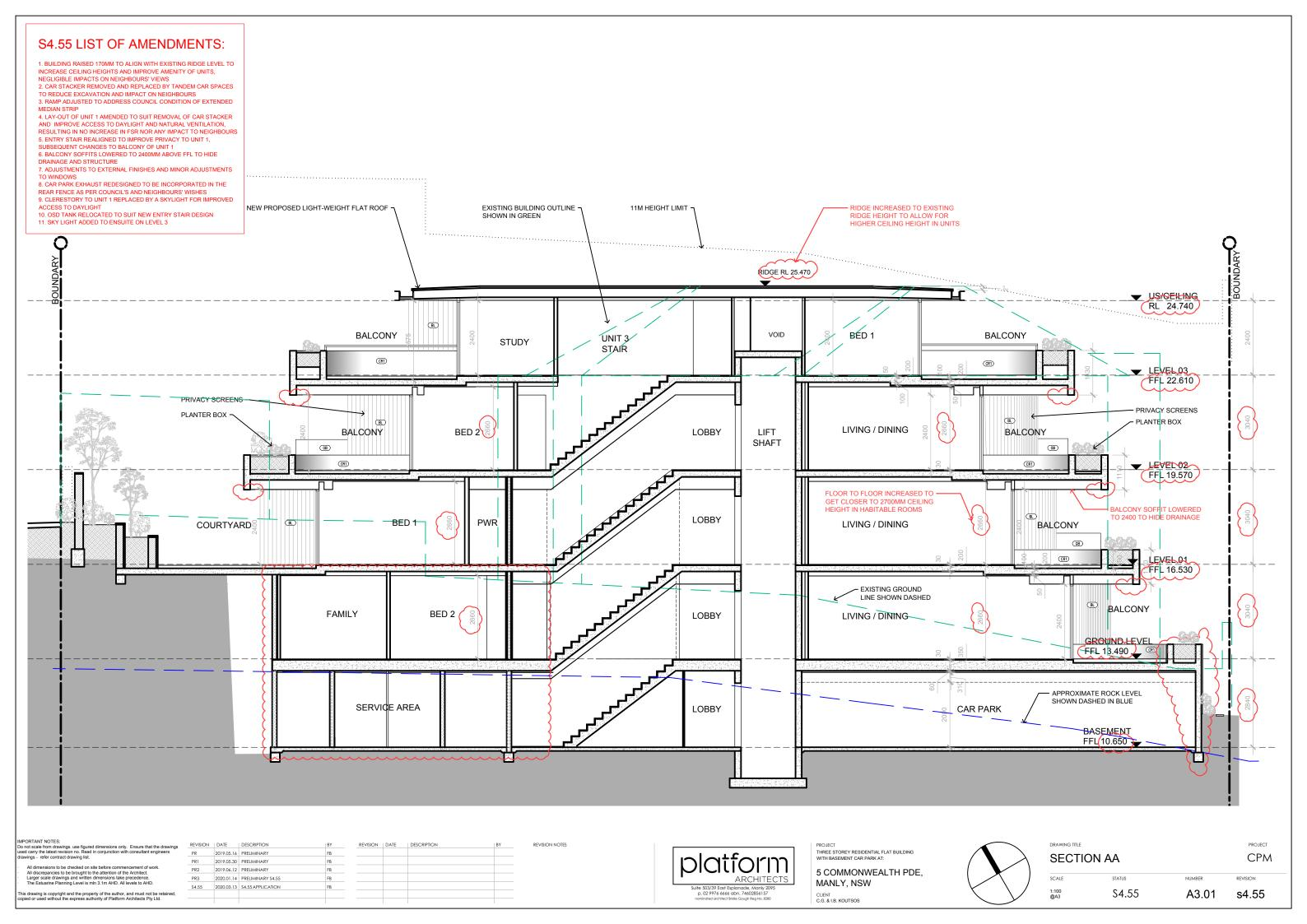
1. BUILDING RAISED 170MM TO ALIGN WITH EXISTING RIDGE LEVEL TO INCREASE CEILING HEIGHTS AND IMPROVE AMENITY OF UNITS, NEGLIGIBLE IMPACTS ON NEIGHBOURS' VIEWS 2. CAR STACKER REMOVED AND REPLACED BY TANDEM CAR SPACES TO REDUCE EXCAVATION AND IMPACT ON NEIGHBOURS 3. RAMP ADJUSTED TO ADDRESS COUNCIL CONDITION OF EXTENDED MEDIAN STRIP MEDIAN STRIP
