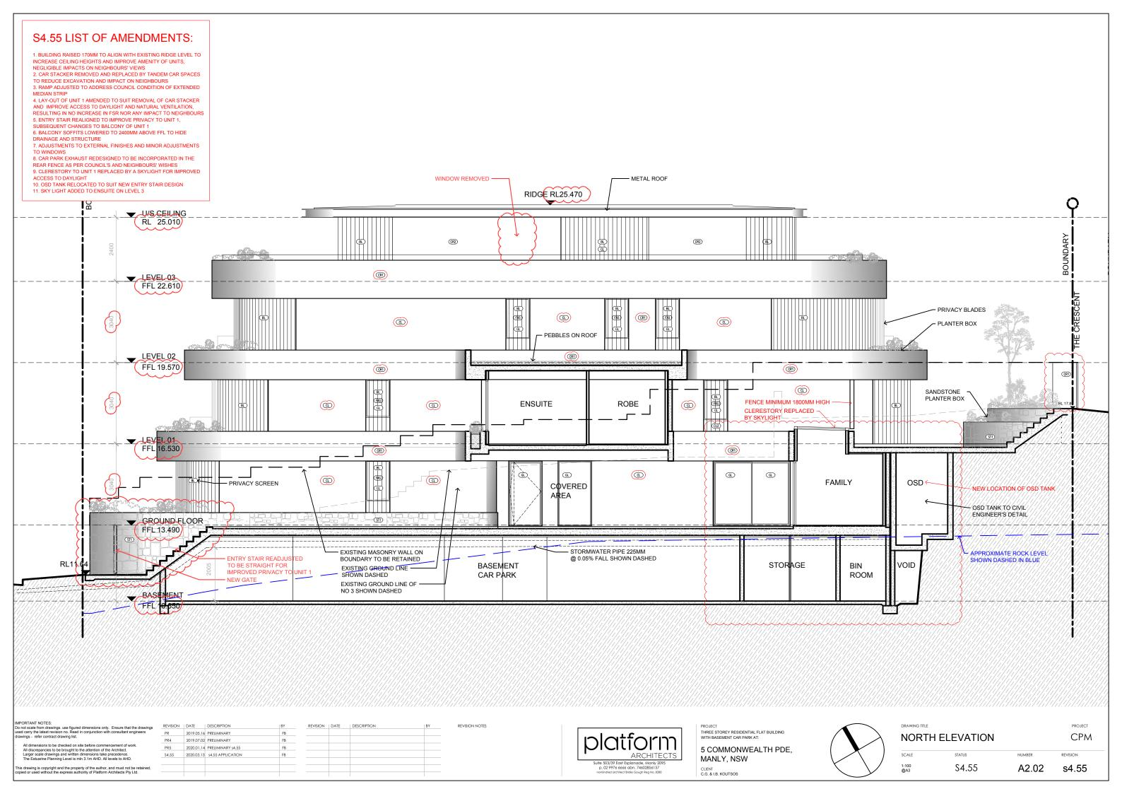
1. BUILDING RAISED 170MM TO ALIGN WITH EXISTING RIDGE LEVEL TO INCREASE CEILING HEIGHTS AND IMPROVE AMENITY OF UNITS, NEGLIGIBLE IMPACTS ON NEIGHBOURS' VIEWS 2. CAR STACKER REMOVED AND REPLACED BY TANDEM CAR SPACES TO REDUCE EXCAVATION AND IMPACT ON NEIGHBOURS 3. RAMP ADJUSTED TO ADDRESS COUNCIL CONDITION OF EXTENDED MEDIAN STRIP
