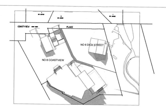
SHADOW AT 3PM MINIMAL IMPACT CDASTVIEV COM VIED SHADOW CAST BY NEIGHBOURS HOUSES AND EXISTING TOPOGRAPHY NO 6 DICK STREET SHADOW CAST BY HOUSE AND EXISTING TOPOGRAPHY
