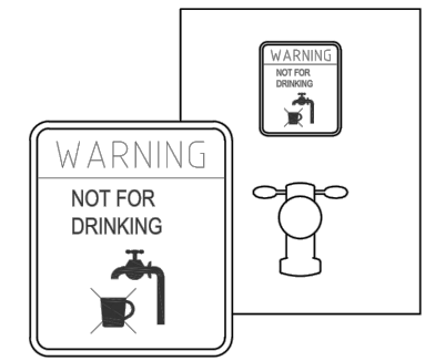
TYPICAL WARNING SIGN SCALE N.T.S * EVERY EXTERNAL SUPPLY OUTLET FROM RAINWATER RE-USE TANK TO BE LABELED WITH METALLIC WARNING SIGN
