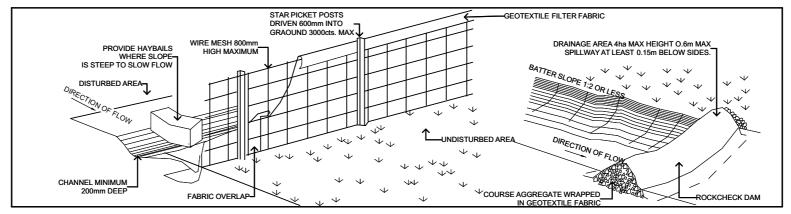
TYPICAL SEDIMENT FENCE SCALE NTS
