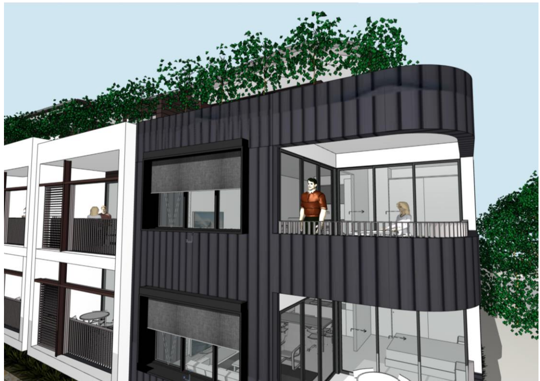
Figure 10: View of west facing units, showing external blinds and balcony overhangs for shading.
