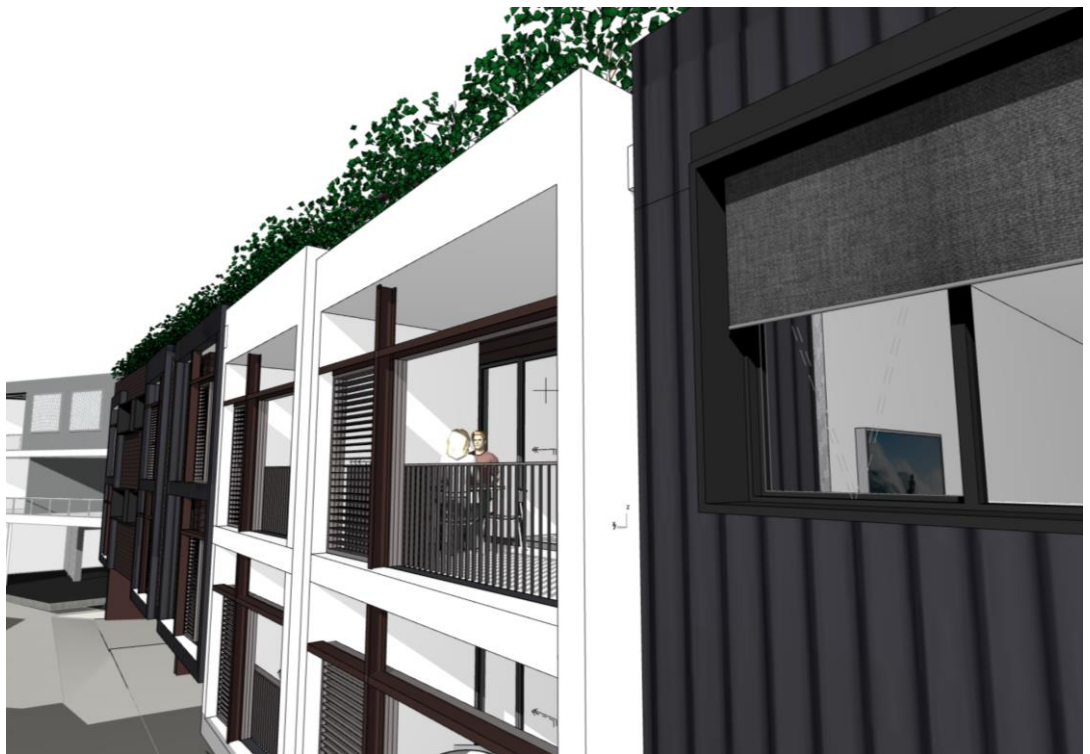
Figure 20: View of operable screens and slatted balustrade on west façade.
