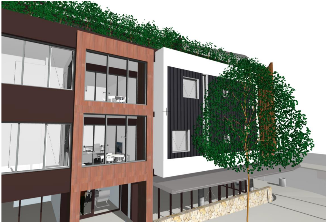
Figure 18: View of corten standing seam cladding on south residential entry portico.
