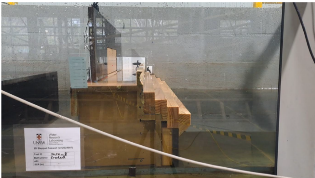
Figure 1 Design 4, 4 bleachers and SLSC wall (eroded profile), recurved parapet
