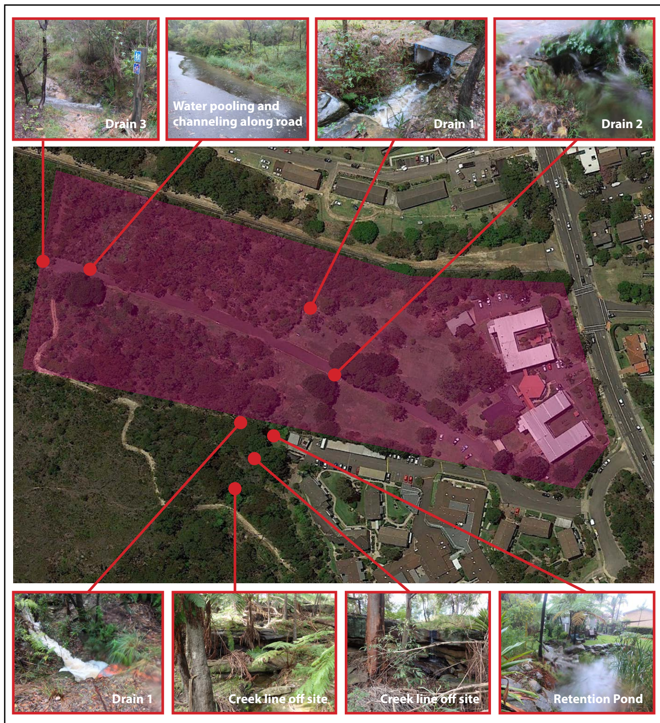
Figure 2. Shows various locations around the site and immediately adjacent to the site on 181 Allambie Rd. Most photos were taken during wet weather in March 2021 and show several drainage points along different drainage lines on the site. Note the rock outcrops and rapid fall off of the creek from the site to the valley below (taken during a dry period).
