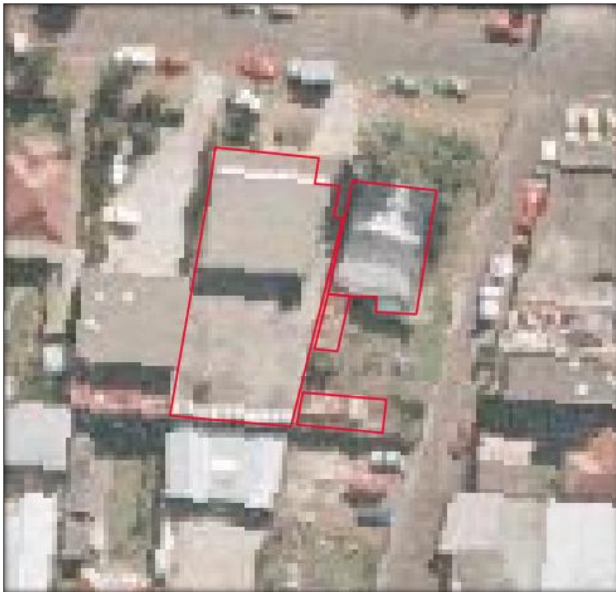
Figure 1: Building footprint used to calculate the existing flood storage (background arial from NSW historical imagery portal, 2005).
