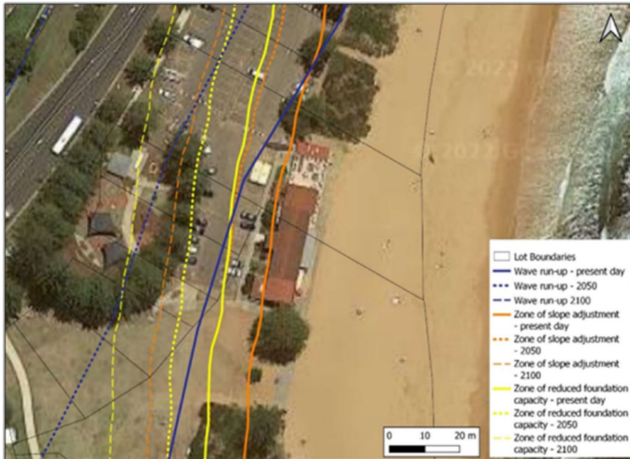
Figure 3-3 Coastal hazard lines (after: Worley Parsons, 2015), aerial image: Google Satellite, 12 March 2018
