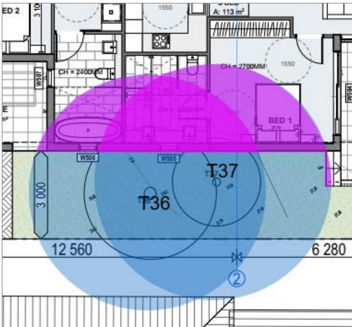
Figure 8 –Tree 36 & 37 encroachment calculation – Excerpt of Level 01 Plan, Project 2306, dwg no. A.06, 23/10/23 authored by Gartner Trovato Architects. Red hashed circle indicates SRZ, blue shaded circle denotes the TPZ. Pink shading indicates encroachment. NOT TO SCALE. Marked up by C Hughes.
