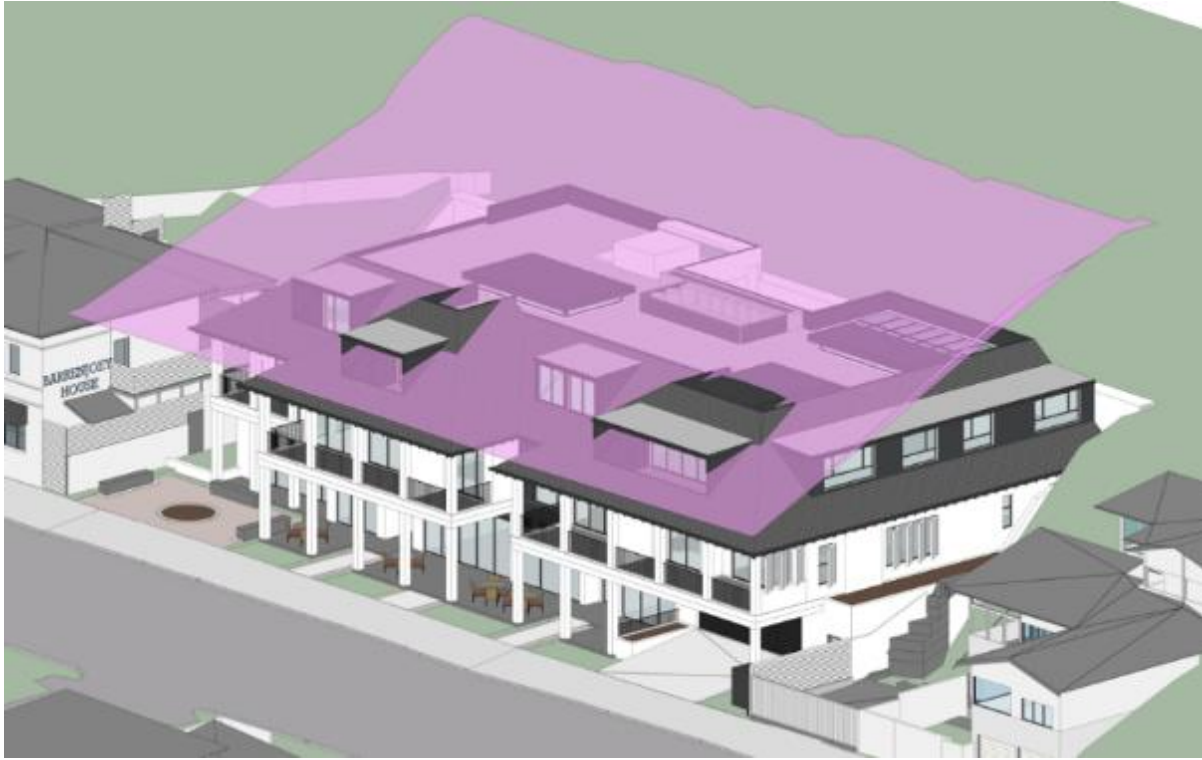
Figure 2 – Interpolated undisturbed building height blanket diagram showing the location and extent of building elements located above the 8.5 metre building height standard.
