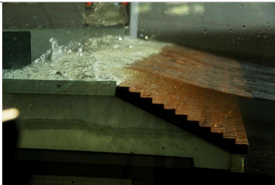
Stepped concrete seawall – 5.45m AHD crest with no wave return wall during 500 year ARI event, present day
