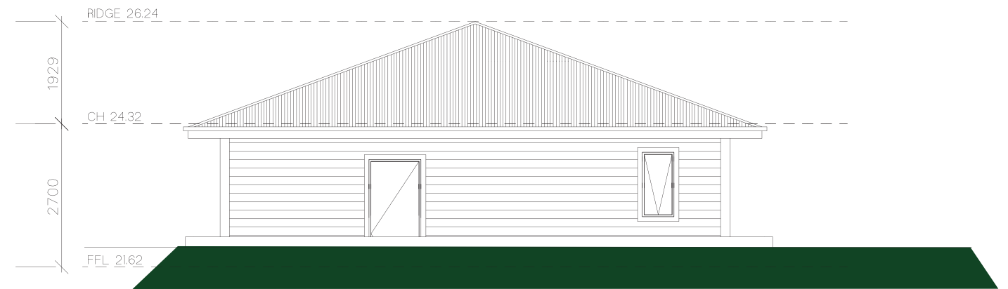
SOUTH WEST ELEVATION 1 : 100
