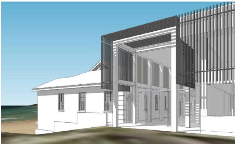
View of MoS building showing alignment of MoS columns with 1935 building engaged piers and windows
