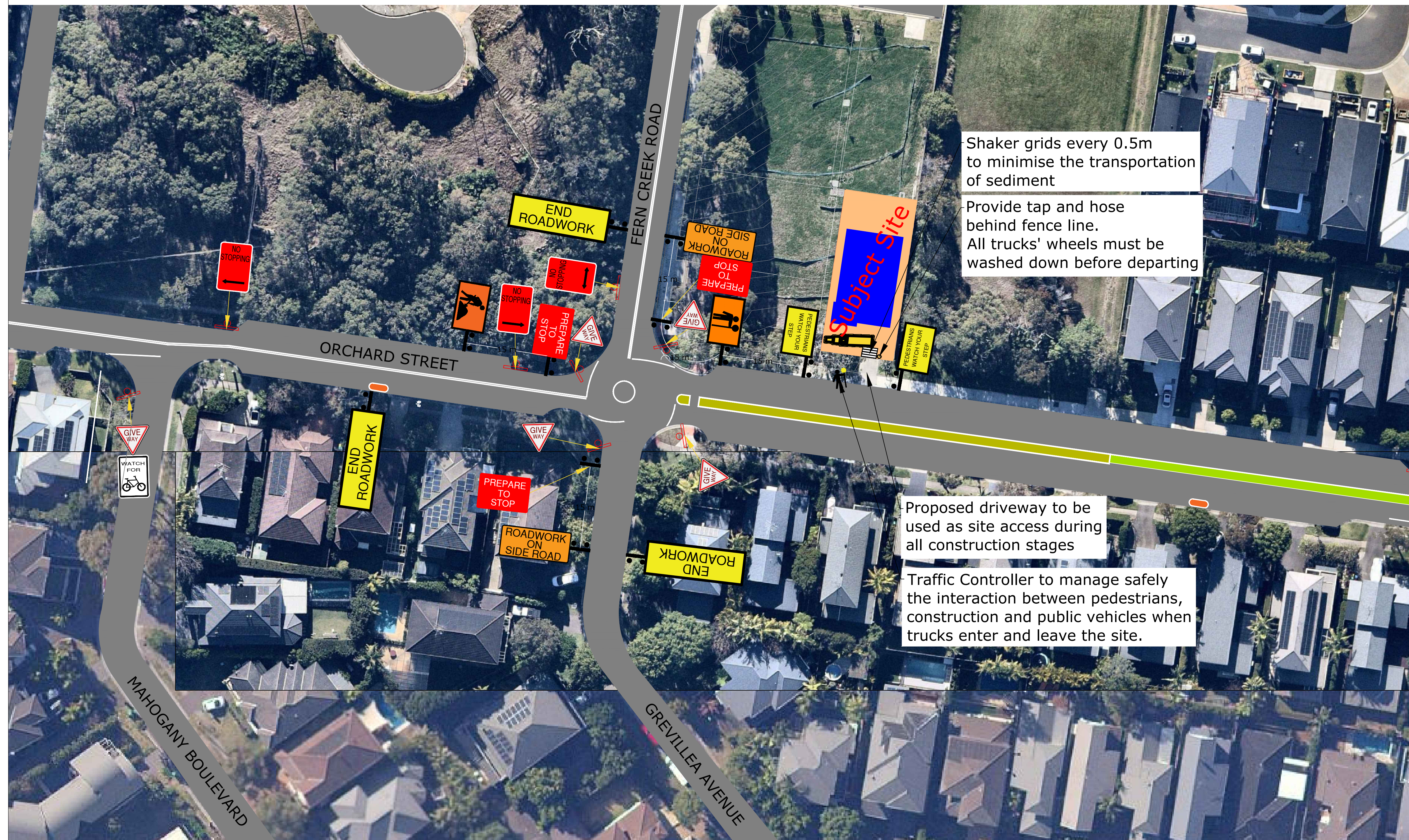
TRAFFIC CONTROL PLAN SCALE 1:400
