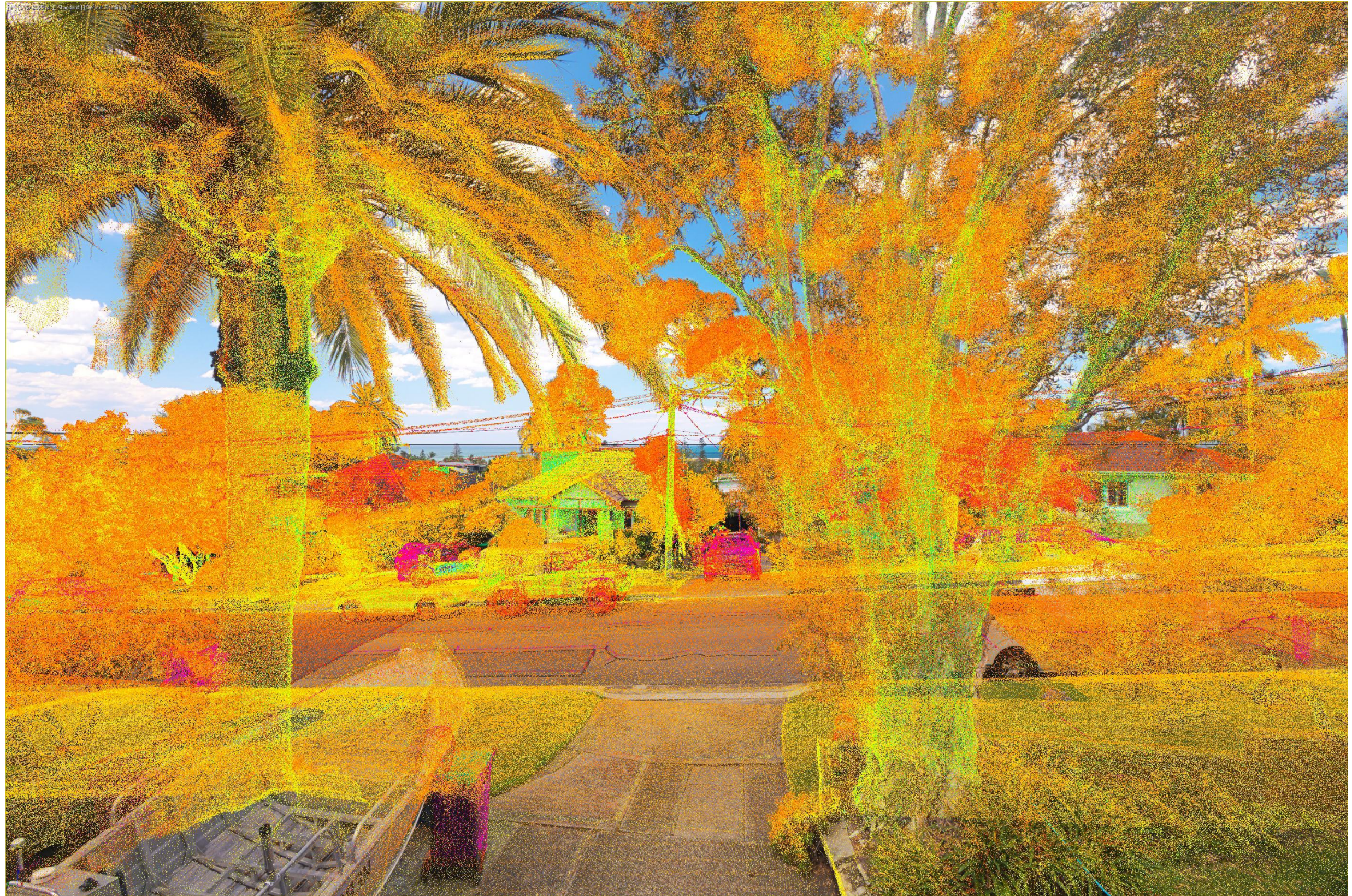
1V5A2065hdr - No.34 : Proof showing surveyed point cloud overlaid on photograph
