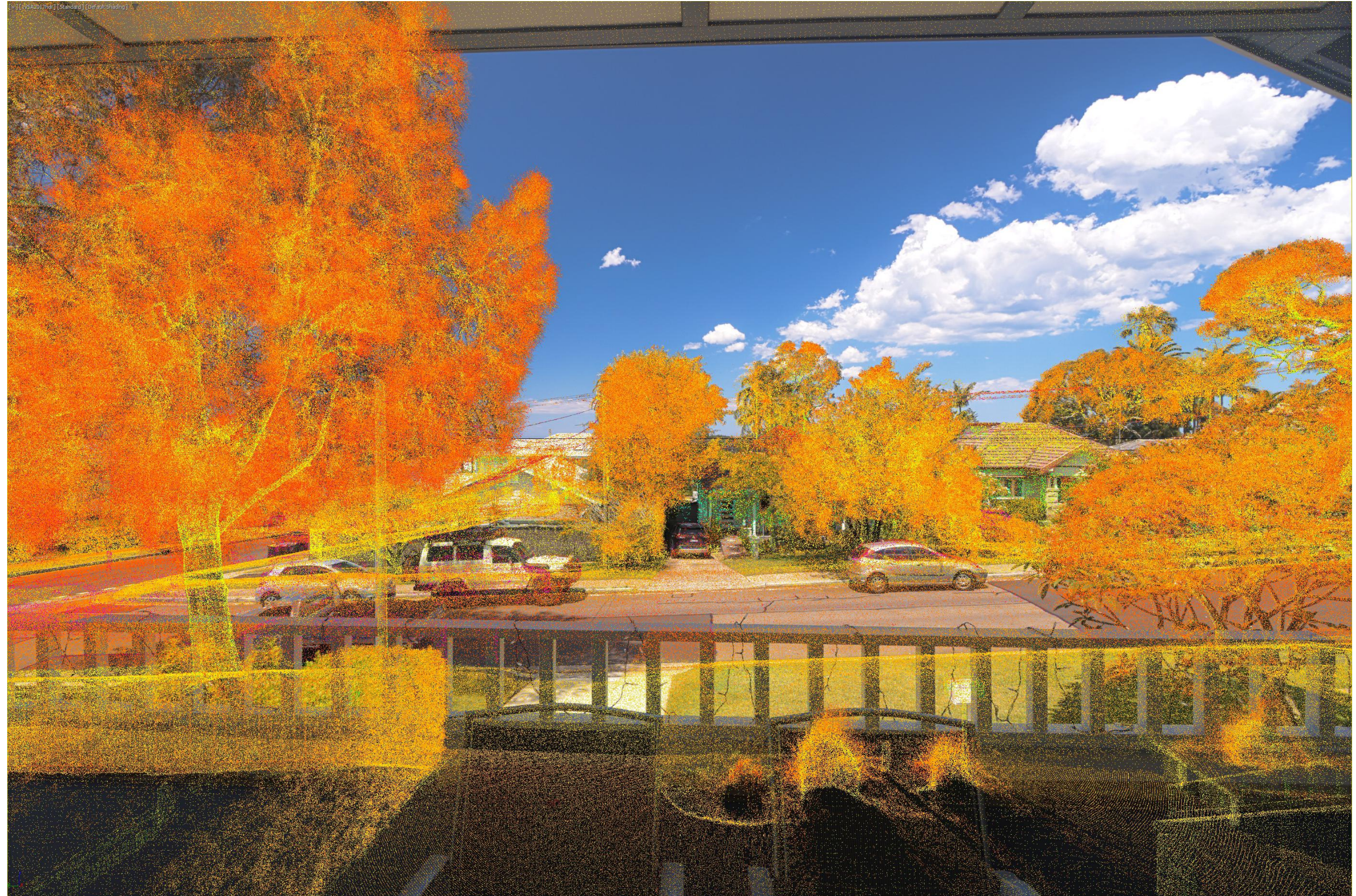
1V5A2017hdr - No.38 : Proof showing surveyed point cloud overlaid on photograph
