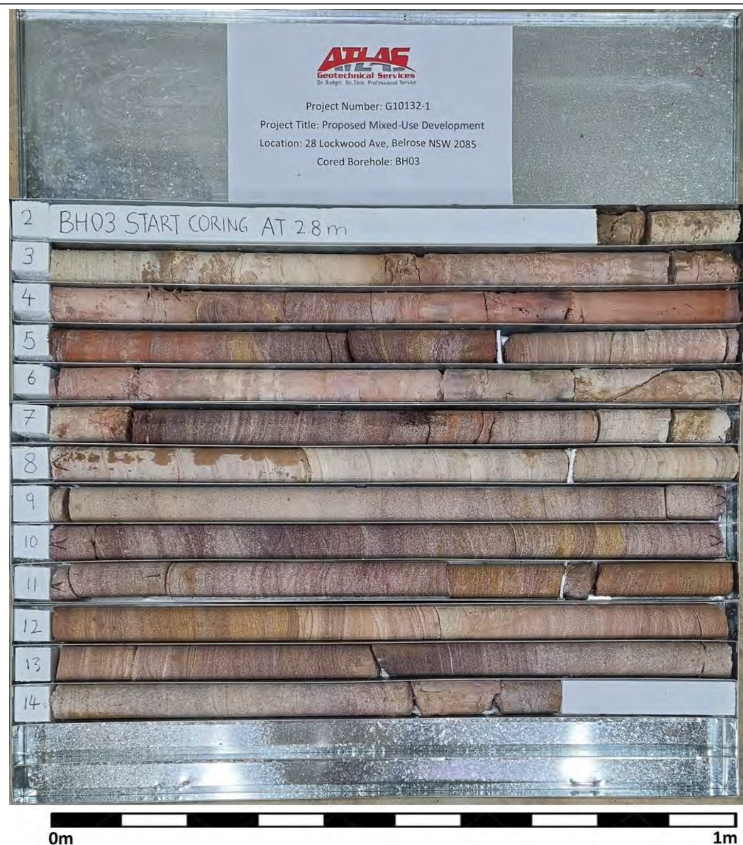
Figure 4.1 – Borehole 3 Core Specimens
