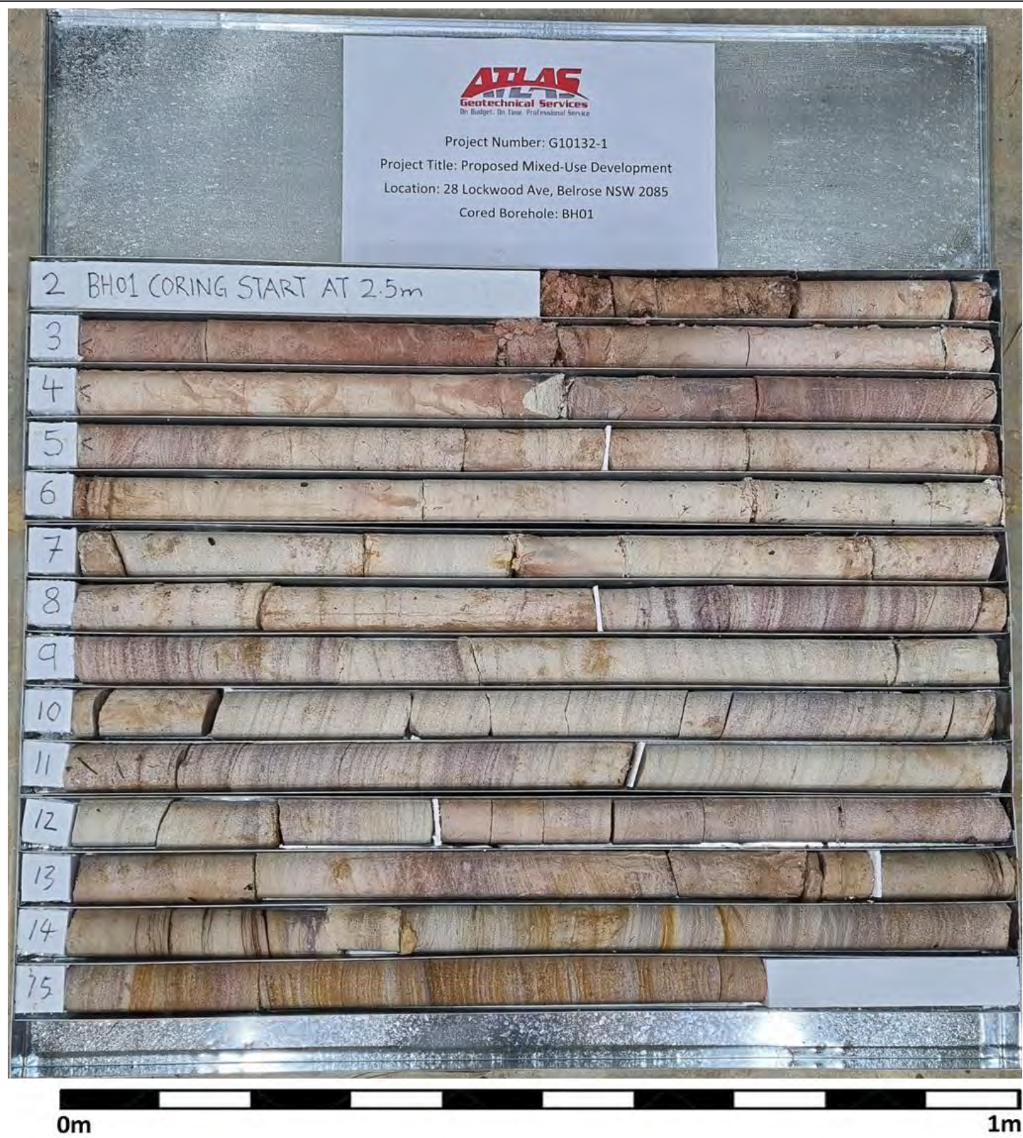
Figure 3.1 – Borehole 1 Core Specimens
