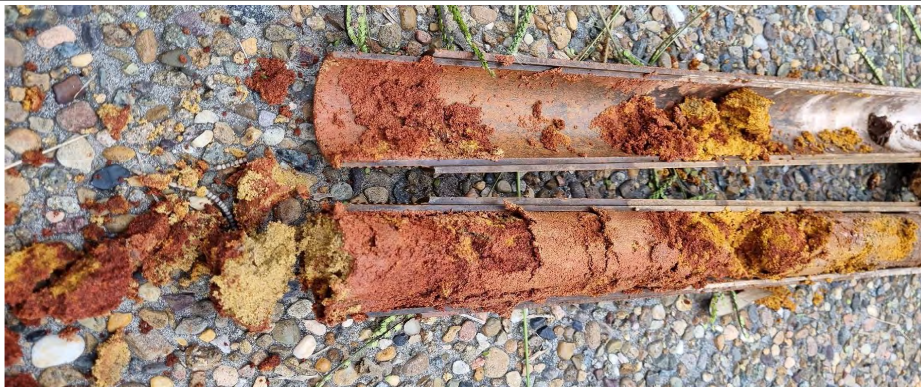
Figure 2.3 – Detail View of SPT Recovered Material (1.0m blg)
