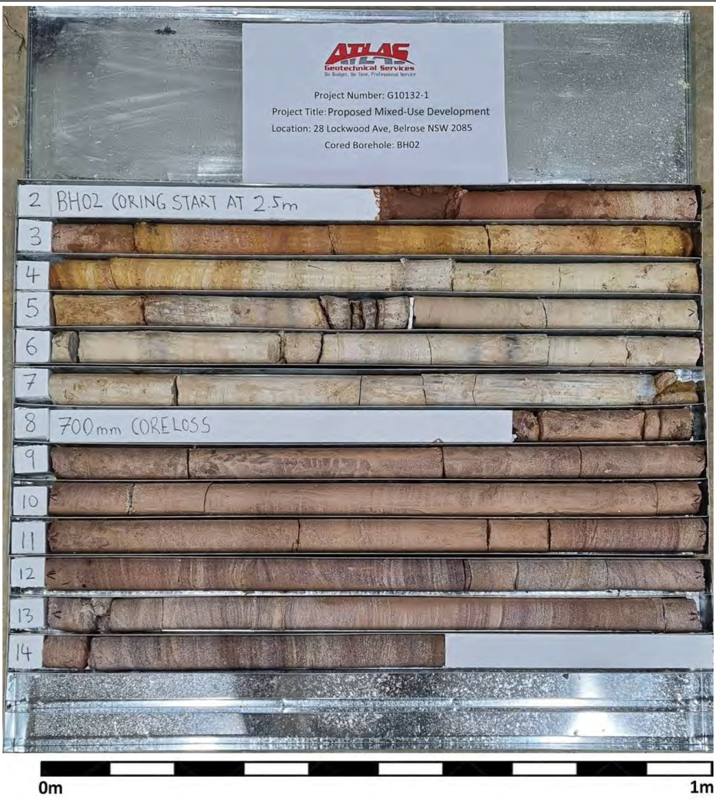
Figure 3.2 – Borehole 2 Core Specimens
