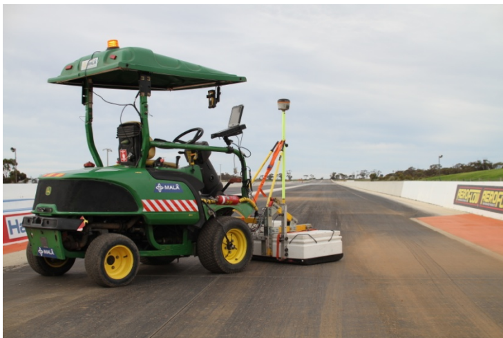
Figure 7 - MALA MIRA 400Mhz 16 Channel 3D GPR System.
