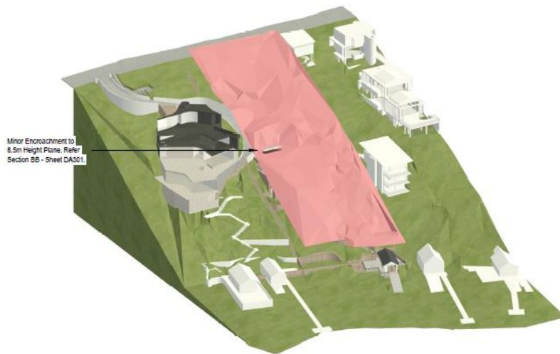
Fig 11: Architectural plan extract to identify the area of the proposed roof to exceed the 8.5m height control (8.95m max height)
