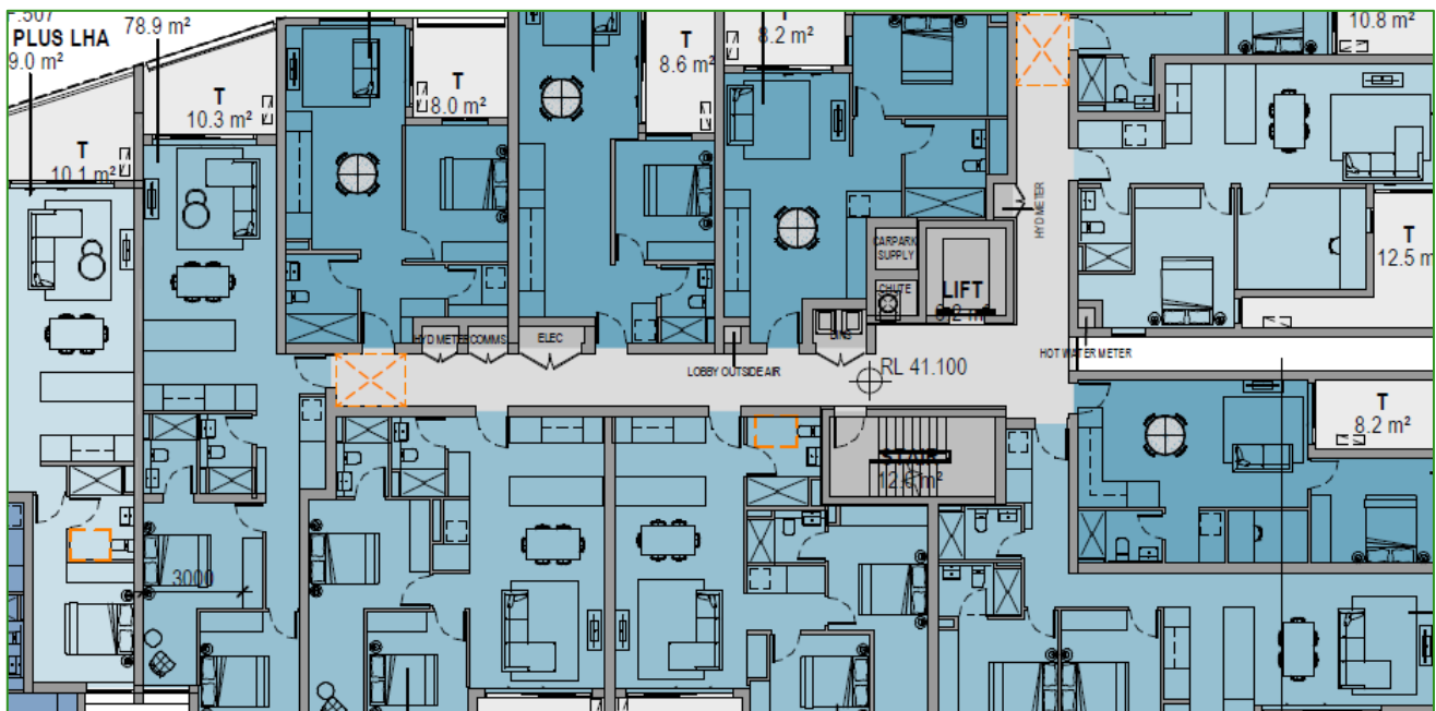
Figure 3 - Waste Chute and Recycling cupboard example
