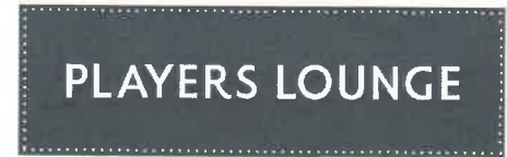
PL01 'Players Lounge' Wall Mounted Lightbox 1125x350mm Lightbox with push through LED dimensional letters and LED chaser light border, mounted to wall above rear entry.
