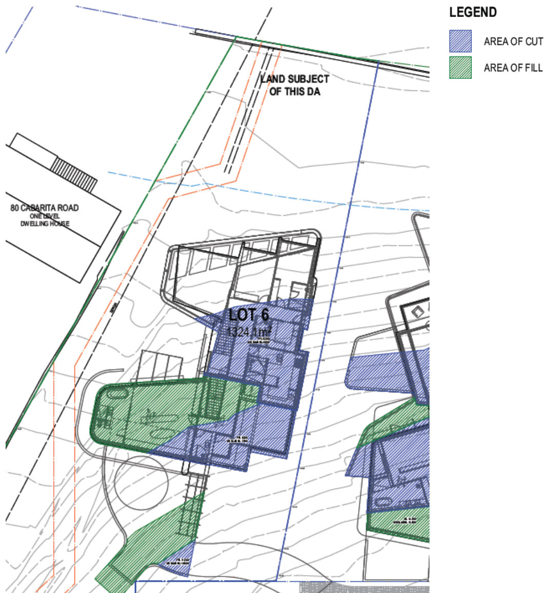
Figure 24 – areas of proposed cut and fill
