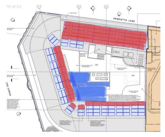
**Image 16:** From master plan, page 10. Solar panels highlighted in red request to remove from design and area in blue add panels below RL/parapet angled towards the beach and screening added below the RL/parapet.
