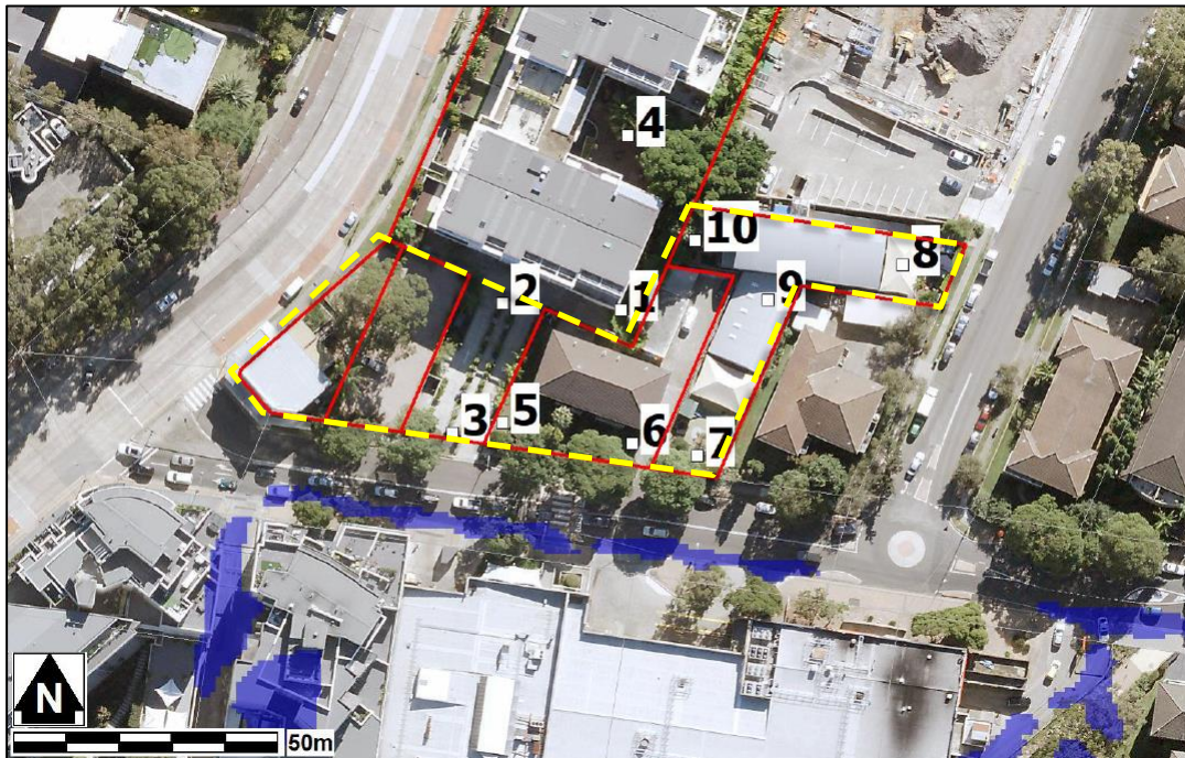
Figure 4 - Extract from Flood Information Report issued by Northern Beaches Council showing 1% AEP flood extent
