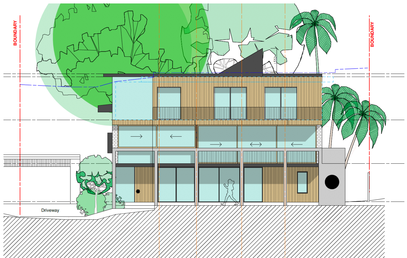
Figure 1 – Demonstrating the very minor non-compliance (shown with blue line) with the building height control.
