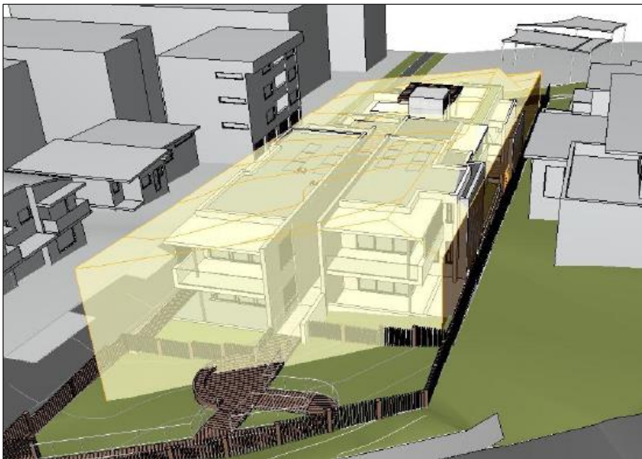
Figure 1 – Building envelope diagram showing limited extent of variation at the western boundary.
