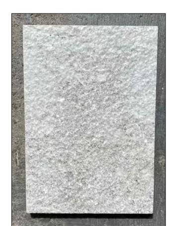
example of 600x300 vitrifed floor tile for balcony and proposed new enclosed room on existing balcony (non slip finish for external area tile)
