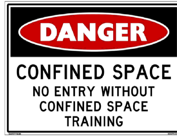
DETAIL - CONFINED SPACE SIGN TO BE PLACED INSIDE OSD TANK & BASEMENT PUMPOUT PIT NTS
