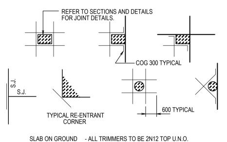
SUSPENDED SLAB - ALL TRIMMERS TO BE 3N16 T&B U.N.O. TYPICAL TRIMMER DETAILS AT ALL COLUMNS, WALLS, PITS, FLOOR WASTES, ETC THAT CAUSE A PENETRATION THROUGH THE SLAB.
