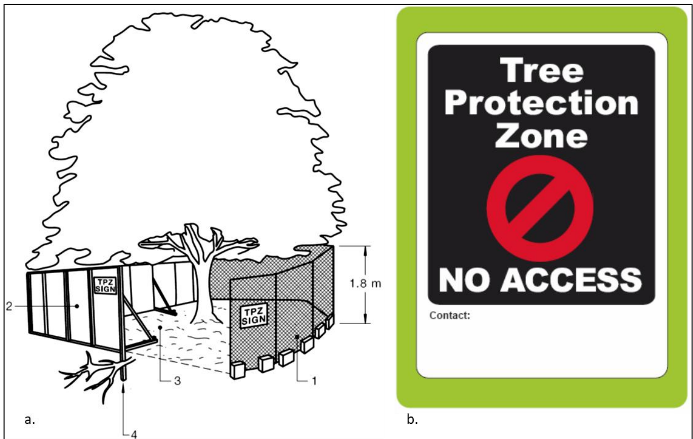
Figure 8. Protection fencing should be erected around the specified perimeter of TPZs in accordance with Section 4.3 of AS4970 (2009) . Figure 8 a. depicts correctly installed steel or plywood fence panelling (1 and 2) with mulch inside the protection area (3). Figure 8 b. shows depicts protection fencing signage.
