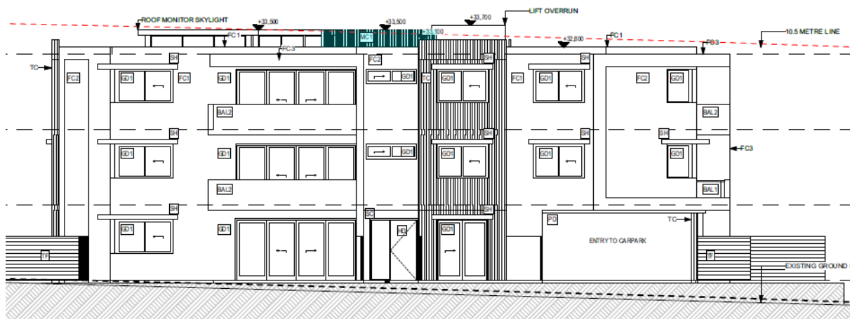
Figure 1 - Plan extract of Building A showing a minor 200mm breach of the building height standard by the proposed roof mounted plant and associated screening
