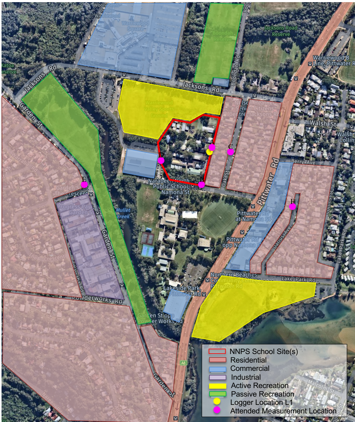
Figure 3: Site Aerial View showing Narrabeen Education Precinct School Site in relation to noise-sensitive receivers, and locations of long- and short-term noise monitoring. Source: Nearmap.
