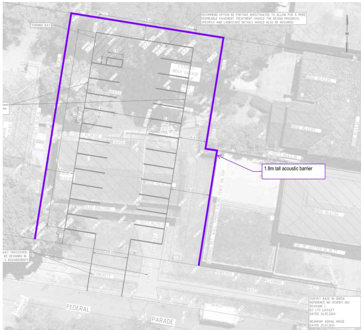
Figure 7: Federal Parade carpark fencing
