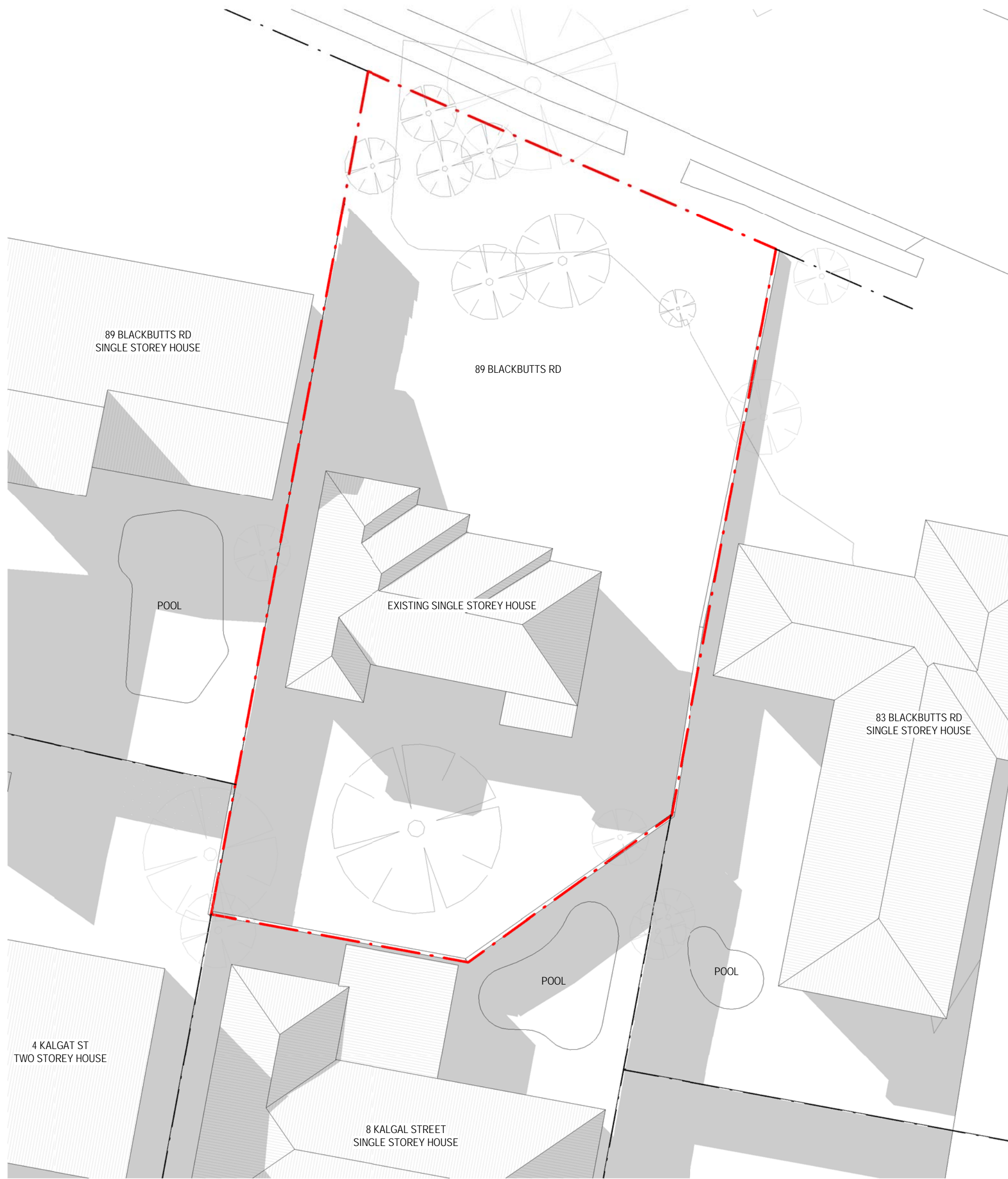
1 EXISTING SHADOW DIAGRAM - 3PM JUNE 21ST DA503 1:200 @ A1
