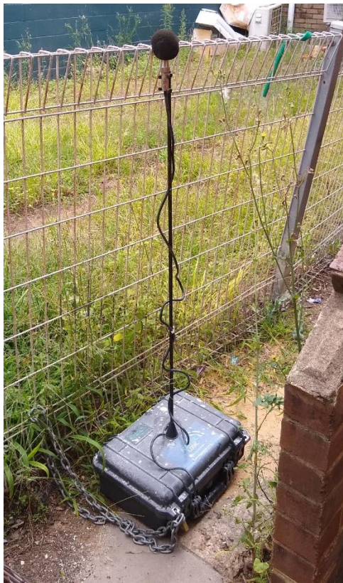
Figure 2 – Noise Monitor Installed on Site
