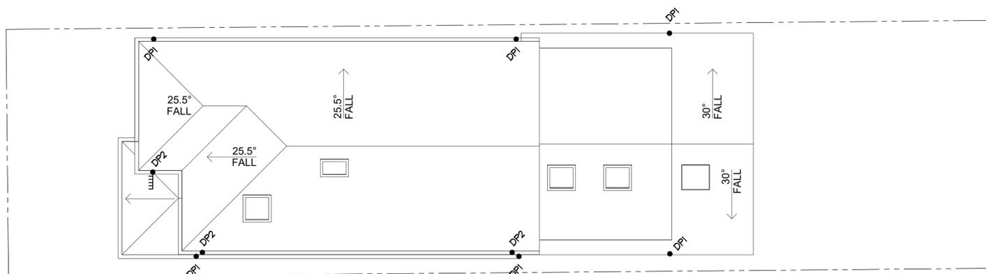
**ROOF STORMWATER DRAINAGE PLAN**
