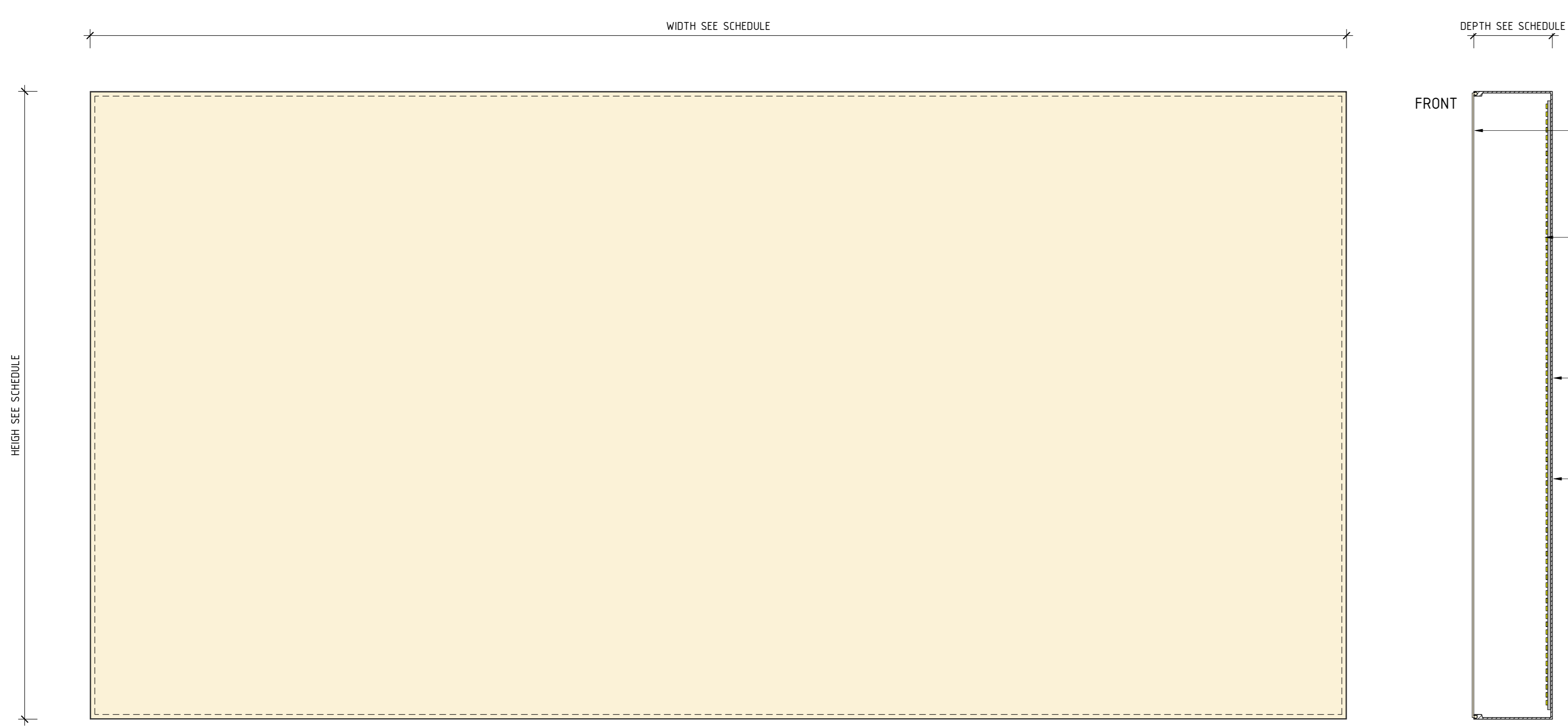
1 TYPE 1 SIGN - TENANT ILLUMINATED SIGN BOX NOTE: THE CHOICE OF TYPE 1 AND TYPE 2 SIGNS DEPENDS ON THE TENANT REQUIREMENT 1 : 10
