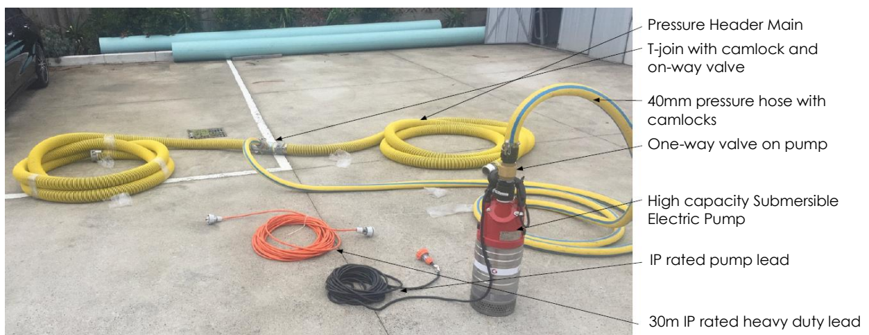
Figure 11-1: Key Components of the Dewatering System
