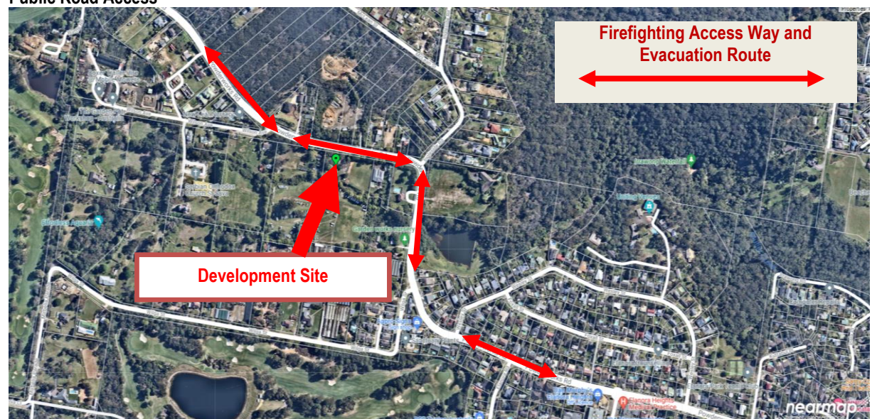
Figure 13 – Access route for fire fighting vehicles and evacuation route for occupants (NearMap 2020)
