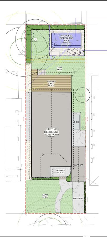
PROPOSED SWIMMING POOL OVERFLOW SHALL BE CONNECTED TO **EXISTING SEWER SYSTEM**
