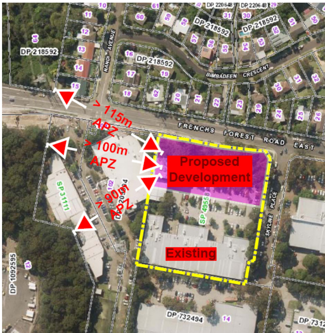
Figure 9 – Cadastre Plan showing the available separation distances to unmanaged Bushfire Prone Vegetation.
