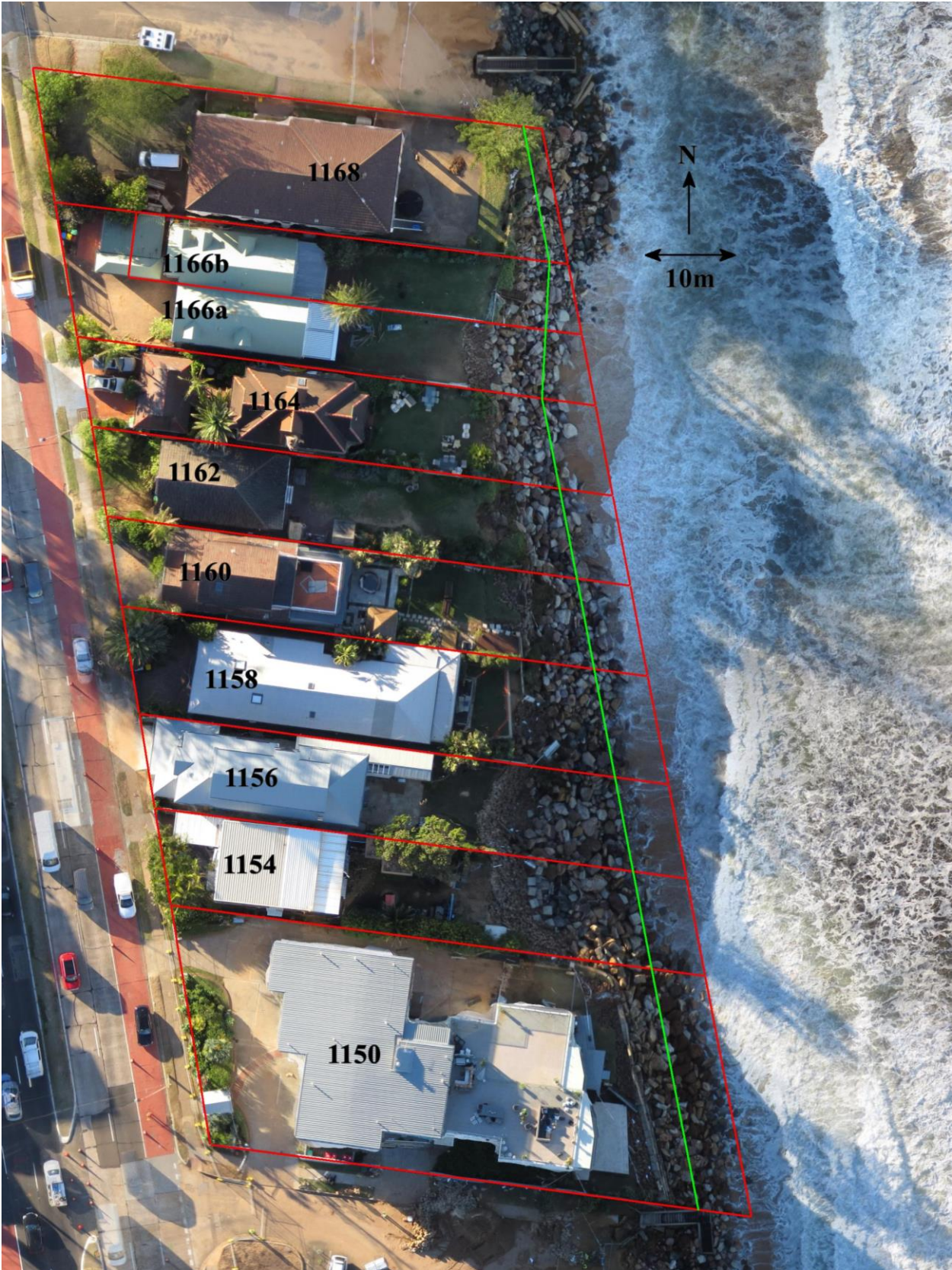
Figure 1: Surveyed boundaries in red, and length of main seawall face in green, at 1150-1168 Pittwater Road Collaroy (aerial photograph taken 8 June 2016)
