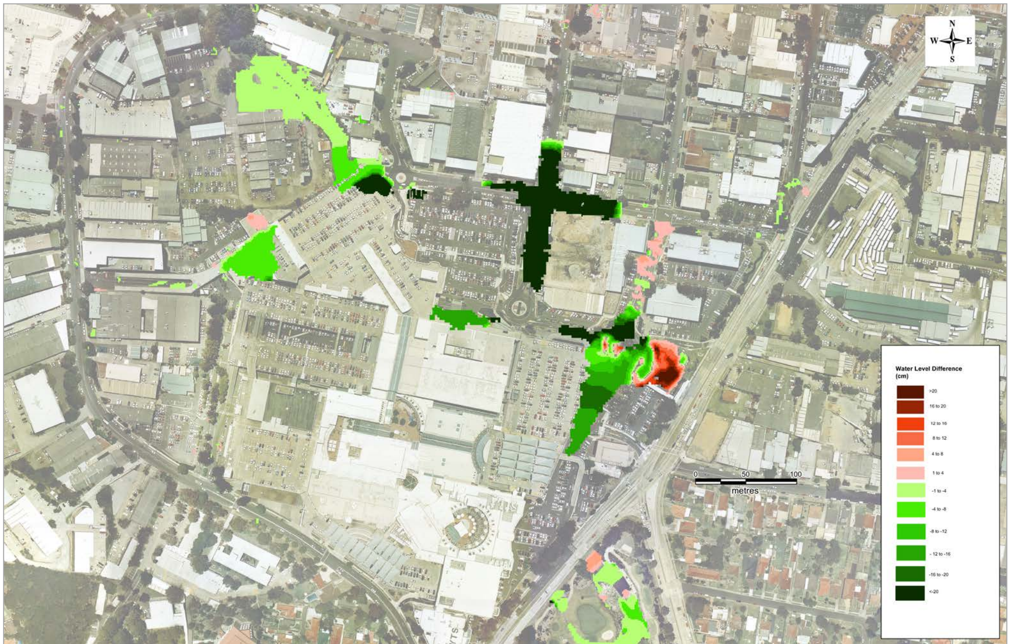
Figure 7A 100 yr ARI Flood Level Differences –DA1514 (2018) Conditions less DA1742 (2015) Conditions - 25% Blockage
