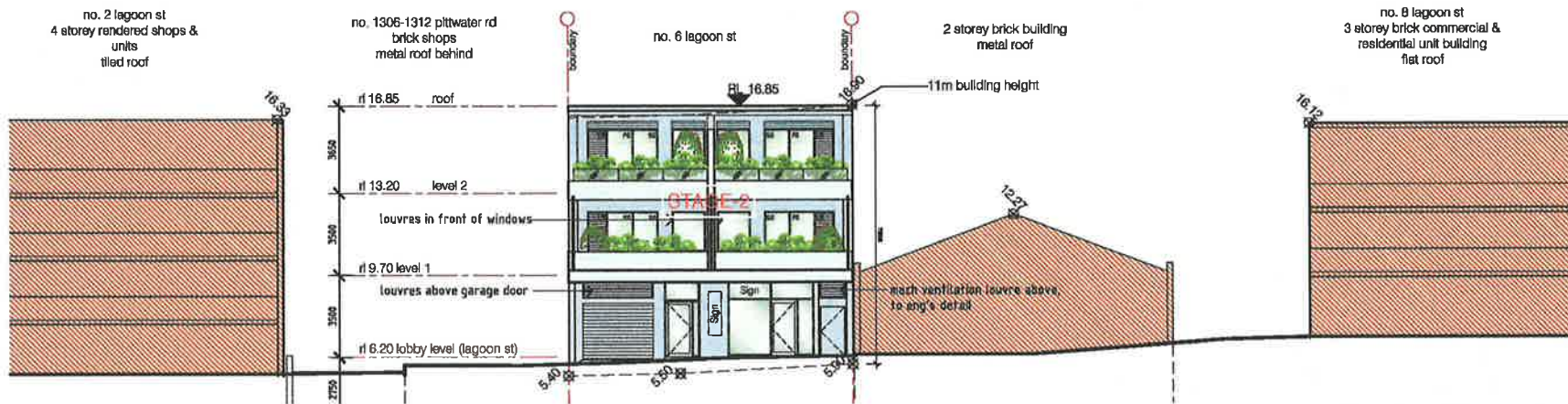
01 EAST ELEVATION (LAGOON STREET) SCALE 1:200@A3
